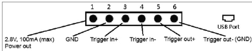
Pin 1: 2.8V, 100mA (max) Power out
